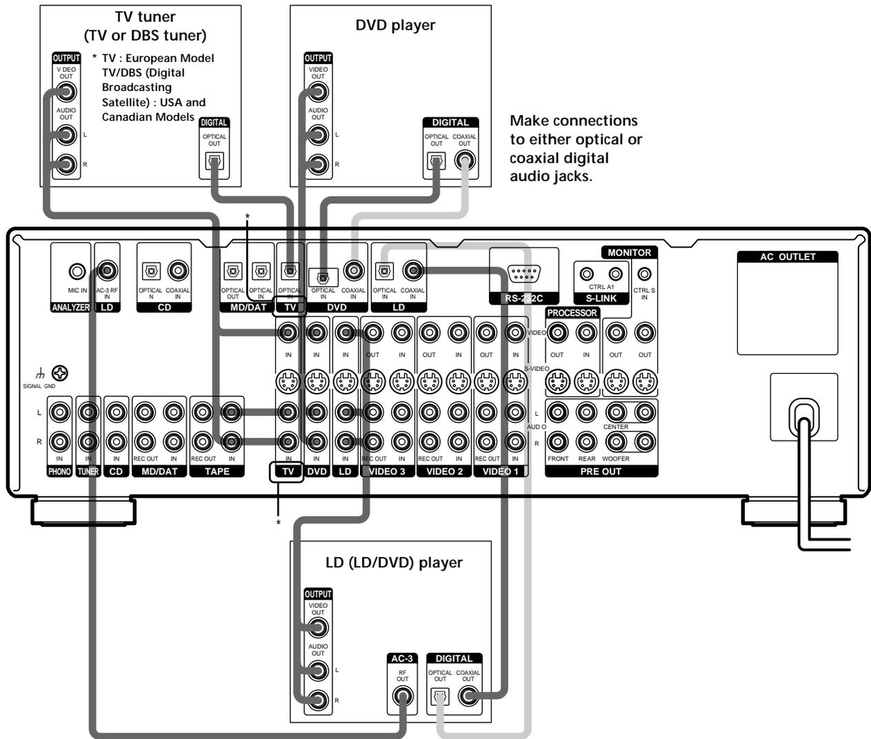
Connect the digital output jack of your MD or DAT deck to the control amplifier's digital input jack and connect the digital input jack of your MD or DAT deck to the control amplifier's digital output jack. These connections allow you to make digital recordings of CDs and TV broadcasts.
